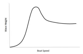
**Figure 4.** Relation of Wave Height to Boat Speed. Source: Oregon State Marine Board (OSMB, 2018).
